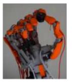
The bionic arm design presented by Mahdi Elsayed Hussein [12] in his thesis project has an impressively low cost of about 250USD weighing 950 grams. The paper talks about a cheap 3D printed bionic arm with 4 grip patterns to perform basic tasks. It also suggest the various improvements that can be made to the model for increasing its functionality. Apart from this the presented arm also has high Finger actuation speed which is quite close to the actual human hand.
